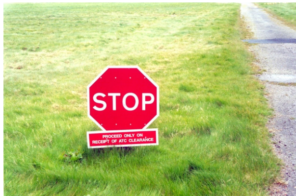
Figure 11-4. Road-holding position sign
